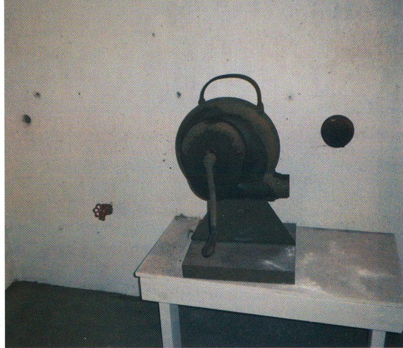
A hand-cranked fan was used to provide air from a vent pipe behind the house with a wall spigot for water.
